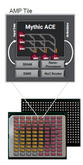
The Mythic Analog Matrix Processor (Mythic AMP™) M1076 integrates a large array of tiles. Source: Mythic.
