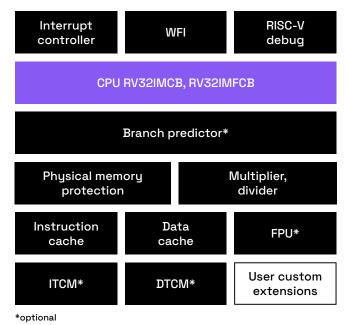
The L31 core can be licensed either as an off-the-shelf (RTL and software toolchain) or fully customizable processor (CodAL).
